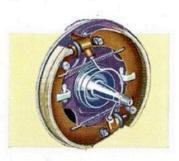
CHRYSLER SAFE-GUARD Hydraulic Brakes—the finest brakes in the Industry. Front brakes have two cylinders per brake, one for each shoe.
